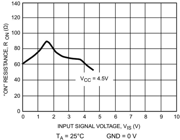
Figure 14-1. Typical ON Resistance vs Input Signal Voltage
