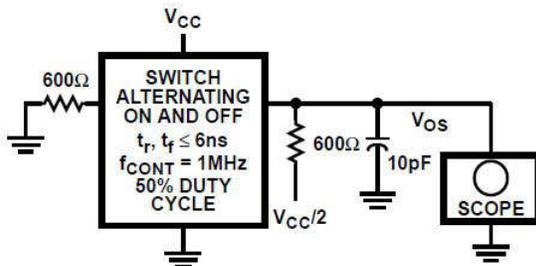
Figure 15-3. Control-to-Switch Feedthrough Noise Test Circuit
