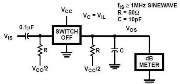
Figure 15-4. Switch Off Signal Feedthrough Test Circuit
