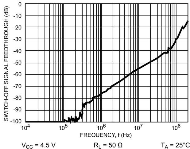
Figure 14-3. Typical Switch-Off Signal Feedthrough vs Frequency
